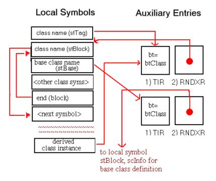
The representation of virtual base classes for C++ relies on the definition of a special symbol that identifies the virtual base table. The name for this symbol is derived from the name of the class to which it belongs. For example, the virtual base table symbol for class C5 would be named "\_btbl\_2C5". This table contains entries for base class run-time descriptions.
