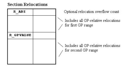
If a section requires an optional relocation entry overflow count, it must be in the first relocation entry.
