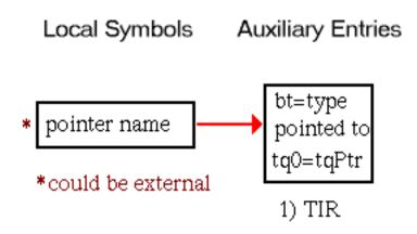
The combination of type qualifiers tqFar and tqPtr are used to represent a short (32-bit) pointer. This pointer type is used with the XTASO emulation.
