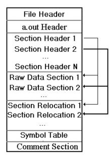
Note that the ordering of section headers does not necessarily correspond to the ordering of raw data and section relocation information. Consumers should rely on the section header to access this information.
