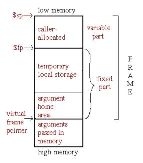
For both types of stack frames, the value of PDR.frameoffset is the size of the fixed part of the stack frame. In the case of a fixed-size frame, it is the entire frame size. For a variable-sized frame, the entire frame size cannot be determined from the symbol table. The code may dynamically increase and decrease the size of the frame multiple times during procedure execution.
