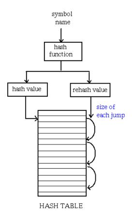
The hash function produces two values for any name it is given: a hash value and a rehash value. The hash value is used for the first lookup. If the symbol found is not the right one, the rehash value is used for chaining. The chain is followed until the correct symbol is found or until the search returns to the symbol where it began.
