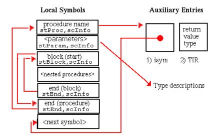
A procedure with no code can contain only nested procedures that also have no code associated with them. If a procedure with no code does not contain any nested procedures, the stBlock/stEnd symbol pair can be omitted from the representation.
