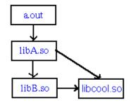
Although the possibility of duplicate dependencies exists, as in the preceding example, each library is mapped only once with the image. The linker also prevents recursive inclusion, which could occur in a case of cyclic dependencies.
