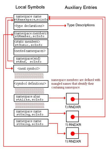
A namespace definition may exist only at the global scope or within another namespace. The namespace representation in Figure 11–7 shows a single contribution to a namespace. This representation may be replicated many times in the symbol table for a single namespace. A namespace definition may be continued within the same file or over multiple source files.
