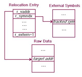
For an external entry, the value for relocation is the run-time address of the referenced external symbol. In cases where the symbol is undefined in an input object, it must first be resolved. Figure 4–5 depicts this process.
