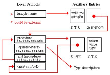
The stProc/scInfo entry has its value set to -2, which distinguishes it from similar entries used to represent procedures with no text and C++ member functions. The stProc/scInfo and stEnd/scInfo entries have null names in the function pointer representation. The parameters are optional and may or may not be named.
