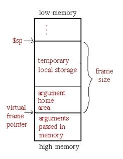
Figure 8–2: Variable-Size Stack Frame
