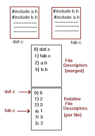
For a symbol reference composed of a file index and symbol index (offset within file), the relative file descriptor table is used as follows:
