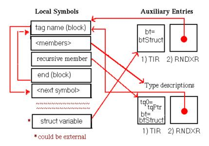
When a field within a structure is itself a structure, the compiler may choose to generate the structure definitions either sequentially or embedded, as shown in Figure 11–28.
