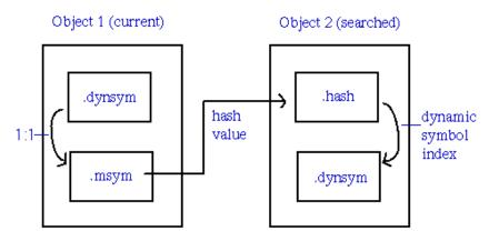
If the .msym section is not present in a shared object, the loader will create the table each time that the object is loaded. For this reason, it is often preferable to specify the .msym section's inclusion when building shared objects.
