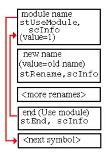
Figure 11–12 shows the representation of a USE statement that imports selected symbols from a module. Note that the stUseModule symbol index field is the index of the local symbol table entry following the corresponding stEnd symbol
