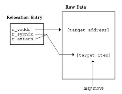
Note that a many-to-one relationship may exist between relocation entries and target items. A target item may be addressed multiple times in an object file's raw
