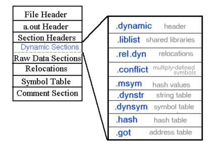
These sections are mapped with the text segment, except for the .got section, which contains the GOT (Global Offset Table). The GOT is part of the data segment because it must be written into when addresses are updated.
