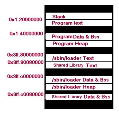
The stack is used for storing local variables. It grows toward zero. The stack pointer (stored in register sp) points to the top of the stack at all times. In generated code, items on the stack are often referenced relative to the stack pointer.
