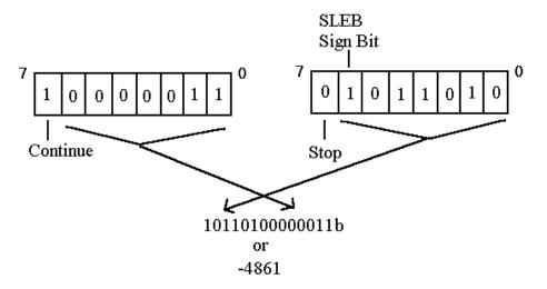
A value represented in LEB 128 format may be signed (SLEB) or unsigned (LEB). The second-highest bit in the final byte of an SLEB value is the sign bit. This means that the signed value has to be propagated only within one byte.
