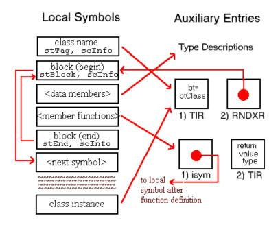
Class members, including member functions, have auxiliary references that point to their type descriptions. Note that member functions are represented as prototypes. The set of symbols defining the member function is elsewhere in the symbol table. To locate the definition of a member function, a name lookup can be performed using the mangled name of the member function with its class name qualifier. See Section 13.3.3 for information on name mangling.
