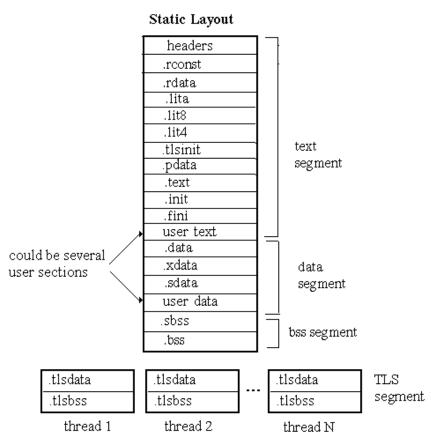
The .rdata and .tlsinit sections are shown as part of the text segment. However, it is possible that one or both of those sections might be in the data segment. They are placed in the data segment only if they contain dynamic relocations.
