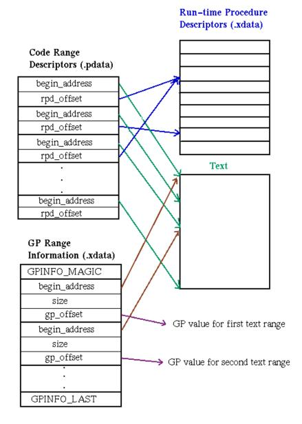
The virtual address space containing the text section of the object file is portioned into code ranges. Each code range descriptor has only one address, which indicates the beginning of the range. The range is implicitly ended just prior to the beginning address of the subsequent range. The final code range descriptor serves to end the range begun by the next-to-last descriptor, not to start a new range.
