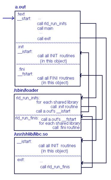
For static executables, the first call is to the main object's \_\_istart() symbol instead of rld\_run\_init(). The dynamic loader is not involved.
