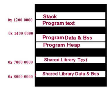
A TASO shared object is marked as such with the RHF\_USE\_31BIT\_ADDRESSES flag in the DT\_FLAGS entry in the dynamic header. The loader recognizes dynamic executable objects marked with the TASO flag and maps their shared library dependencies to the TASO address space. A TASO static executable is not explicitly identified in object file structures.
