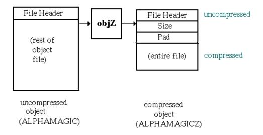
The value of "size" is the size of the uncompressed object in bytes. The archiver uses the "pad" value to indicate the bytes of padding it inserted. Both fields are 8-byte unsigned integers.
