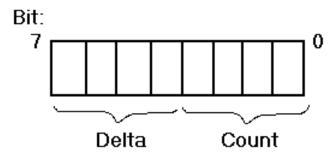
Figure 7–2: Line Number Byte Format
