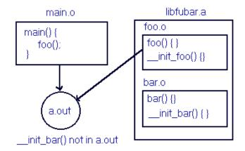
On the other hand, if the archived object is already linked into the object, prefix recognition will apply to routines contained in that module. Explicit inclusion can be used to ensure an archived routine is included as an initialization or termination routine in all cases. See the *Programmer's Guide* for more information on linking with archive libraries.
