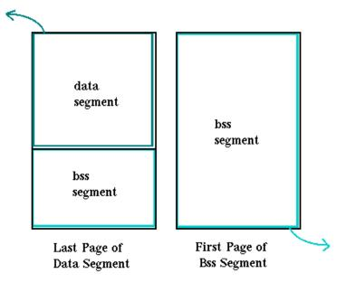
When part or all of the bss segment is contained in the last page of a data segment, that portion of the data page must be initialized to zero in the corresponding raw data area of the object file.
