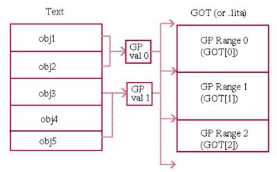
Objects can share a GP range, as shown in Figure 2–7, or use more than one GP range, depending on the amount of program data. However, the *Calling Standard for Alpha Systems* specifies that a single procedure can use only one GP value. The a.out header's gp\_value field contains either the GP value of the object (if there is only one) or the first one the program should use (if there are multiple GP ranges).
