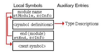
External symbol table entries for declarations contained in modules use a simple form of name mangling. As illustrated in Section 17.3.4, the external name is constructed by converting names to lower case and assembling them as:
