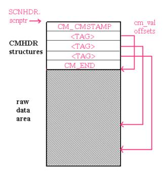
Begin and end marker tags are used to denote the boundaries of the structured portion of the comment section. The begin marker is CM\_CMSTAMP, which contains a comments section version stamp, and the end marker is CM\_END. If either of these headers is missing or the version indicated by the value of CM\_CMSTAMP is invalid, the comment section is considered invalid.
