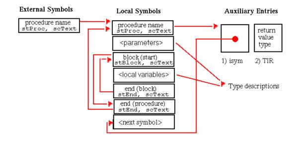
A special instance of a procedure definition occurs for a procedure with no text. This type of procedure occurs only in the local symbol table and is very similar to the representation of other procedures. It is generally used for procedures that have been optimized away that still need to be represented for debugging or profiling information.
