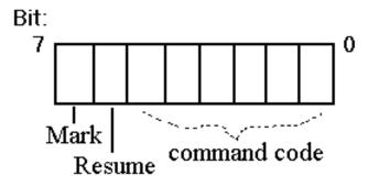
Command parameters are stored in LEB (Little Endian Byte) 128 format. See Section 1.4.6 for a description of this data representation. PC deltas are always expressed as machine instruction offsets and must be scaled by the size of a machine instruction before adding to the current PC. No other deltas need to be scaled.
