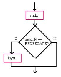
The final step is to decode the RNDXR records. The basic types that are followed by RNDXR records require reference to another local or auxiliary symbol to complete the type description. Interpret the RNDXR records as follows:
