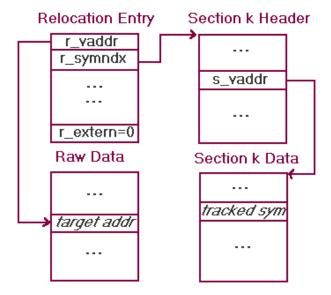
For a local entry, the value for relocation is the difference between a section's address in the input object and the address of that section's data after linking. The section is identified by a relocation section type in  $r_symndx$ . Figure 4–7 depicts this situation.
