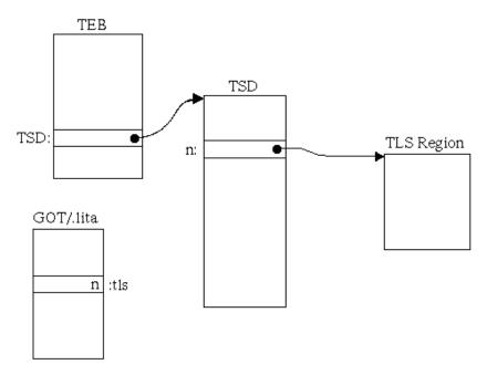
Because the TLS region is allocated dynamically and is unique per-thread, no address information can be recorded in the object file. All other attributes of the TLS region can be determined at link time and are recorded in the object file in the TLS data and TLS bss section headers.
