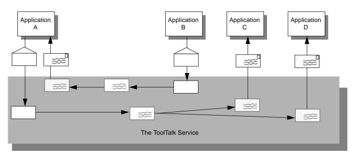
Figure 1-1 Applications Using the ToolTalk Service
