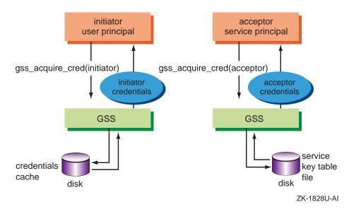
The gss\_acquire\_cred() function uses an imported name to look for a valid ticket associated with the user or service name. The credentials must already exist in the HP credentials cache for the initiator or the service key table for the acceptor. An exception is an acceptor application that also initiates security contexts with other acceptor applications. A common example is a proxy. In this case, both a credentials cache and a service key table file entry is required to support either role.
