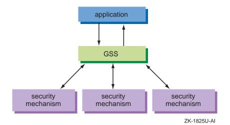
A *security mechanism* is a method of providing security (such as Kerberos or public-key encryption). It is not only the cryptographic technology used, but also the syntax and semantics of the data that the technology employs. An application secured using the GSS-API standard may use one or more security mechanisms.
