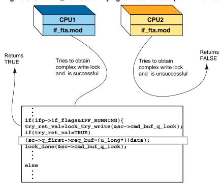
Figure 8-5: The if fta Module Trying to Assert a Complex Write Lock
