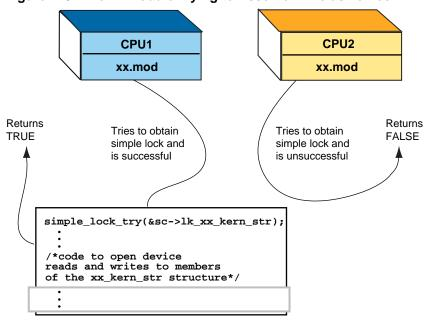
Figure 7-3: The xx Module Trying to Assert an Exclusive Lock
