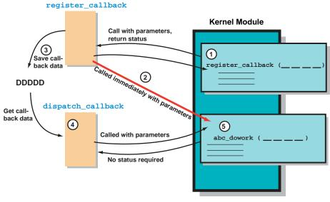
Figure 4-2: Using the Kernel Callback Subsystem
