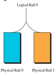
Figure 10-2: Failover Pair Memory Channel Configuration
