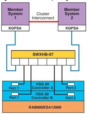
Figure 7-5: Arbitrated Loop Configuration with One Storage Array
