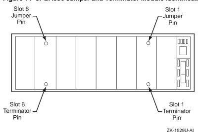
Figure 11-8: BA356 Jumper and Terminator Module Identification Pins
