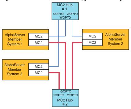
Figure 5-8: MC1-to-MC2 Standard Hub Upgrade: Final Configuration
