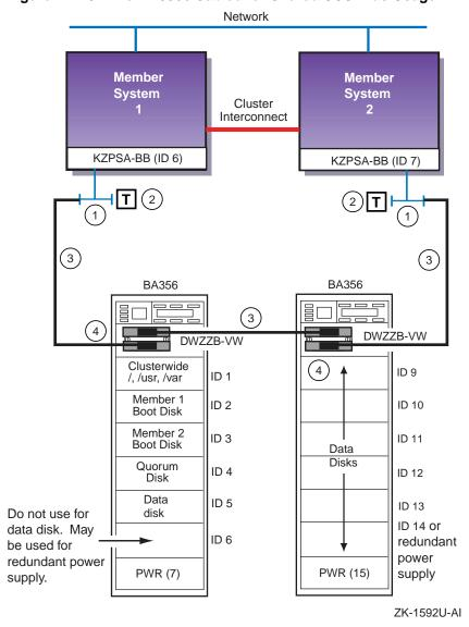
Figure 11-10: Two BA356s Cabled for Shared SCSI Bus Usage
