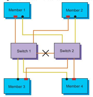
Figure 6-5: Nonrecommended Redundant LAN Interconnect Configuration
