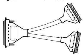
Figure 11-5 shows an HD68 trilink connector (H885-AA), which you may attach to a KZPSA-BB or KZPBA adapter that has its onboard termination removed, or on the unterminated differential side of a SCSI signal converter.
