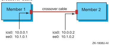
A crossover cable for point-to-point Ethernet connections is required to directly connect the network adapters of two members when no switch or hub is configured between them.
