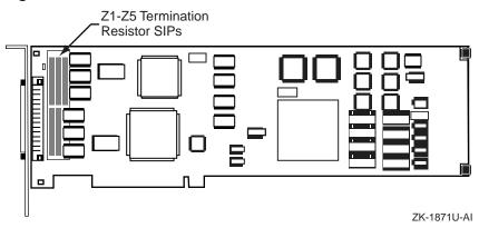
The KZPBA internal termination is disabled by removing the termination resistors RM1-RM8 as shown in Figure 4–1.
