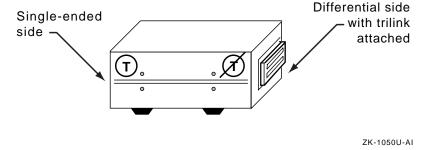
Figure 11–2 shows the status of internal termination for an SBB SCSI signal converter that has a trilink connector attached to the differential side.
