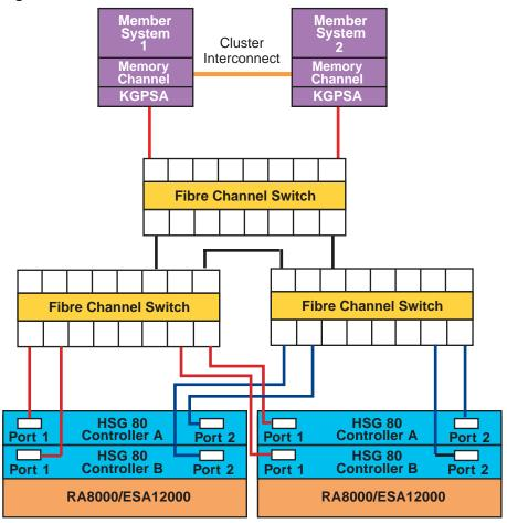
Figure 7-12: Meshed Fabric with Three Cascaded Switches
