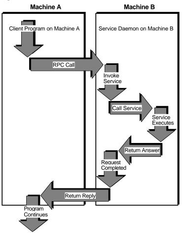
Figure 1–1: Basic Network Communication with Remote Procedure Call
