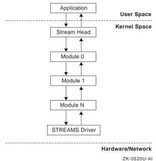
The Stream head is a set of routines and data structures that provides an interface between user processes and the Streams in the kernel. It is created when your application issues an open system call. The following are the major tasks that the Stream head performs:
