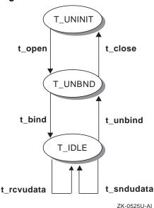
Figure 3-4: State Transitions for the Connectionless Transport Service
