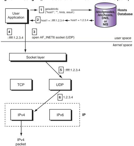
Figure 4-4: Using AF\_INET6 Socket for IPv4 Communications (Send)
