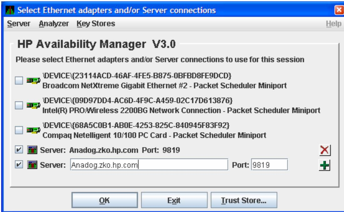
To start the Data Analyzer, clear the checkbox for the last entry. The Data Analyzer then uses the Data Server running on Anadog.zko.hp.com. Figure 7.
