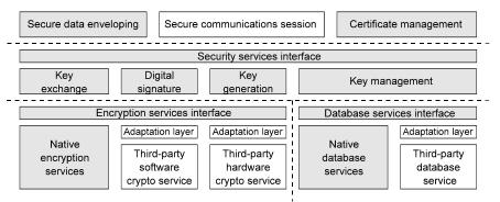
The key database services are implemented as an interface layer which communicates with various key storage technologies and mechanisms. This layer is as follows:
