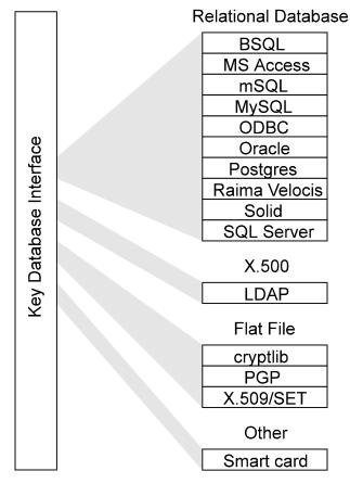
The low-level encryption services are implemented as plug-in modules which can be added and removed as required. This layer is as follows:
