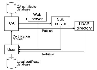
To handle certificate trust and revocation issues, cryptlib includes a certificate trust manager which can be used to automatically manage CA trust settings, for example a CA can be designated as a trusted issuer which will allow cryptlib to automatically evaluate trust along certificate chains. Similarly, cryptlib can automatically check certificates against CRL's published by CA's, removing from the user the need to perform complex manual checking.
