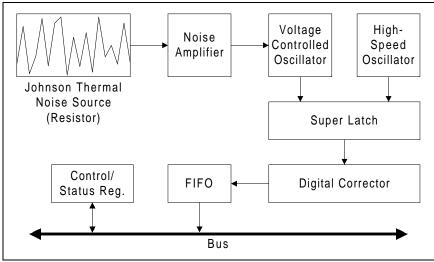
Figure 1: Block diagram of the Intel RNG
