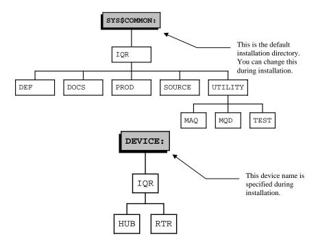
Alternatively, the installation routine can install the SYS\$COMMON files onto a separate device. In addition, a command procedure, IQR\_STARTUP.COM, is created in your SYS\$STARTUP directory.
